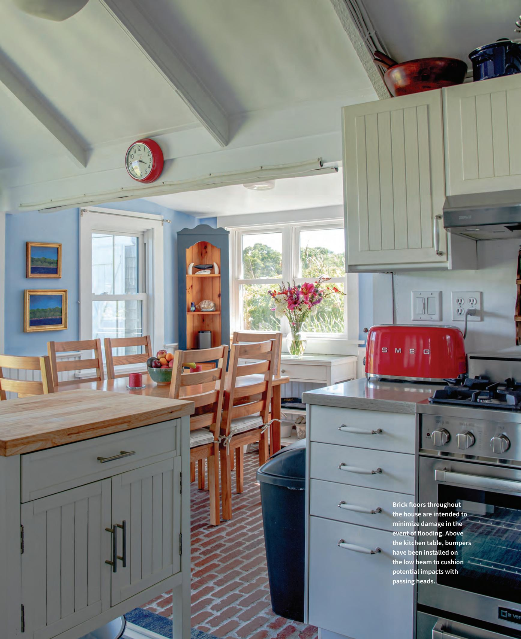
Brick floors throughout the house are intended to minimize damage in the event of flooding. Above the kitchen table, bumpers have been installed on the low beam to cushion potential impacts with passing heads.
